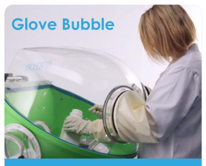
The Glove Bubble is a bench mounted enclosure designed to provide a sealed environment for samples as well as offer control of atmospheres internally.
